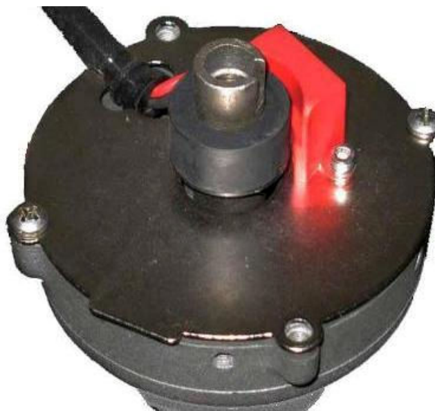
Example of a Hot-Spark kit in a Delco non-vacuum-advance distributor
